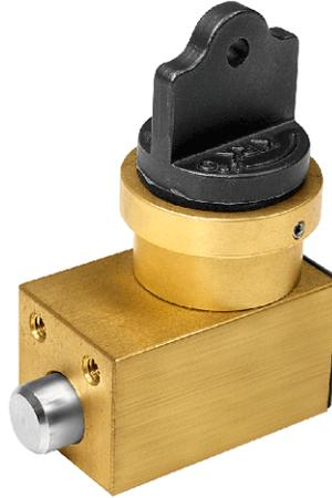
The Type FN interlock has a more narrow housing than the Type F interlock and is mounted by means of 1/4"-20 tapped holes in the end of the housing. The interlock housing is made from brass. The key, lock bolt and all internal parts are constructed from 316 stainless steel. The lock bolt is 5/8" diameter and the throw, or travel, of the lock bolt is 3/4". Lock bolt movement is completely controlled by the rotation of the key.
